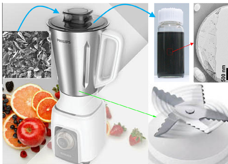
Fig. 1 – The schematic of a kitchen blender for preparing FLG flakes. (A color version of this figure can be viewed online.)
